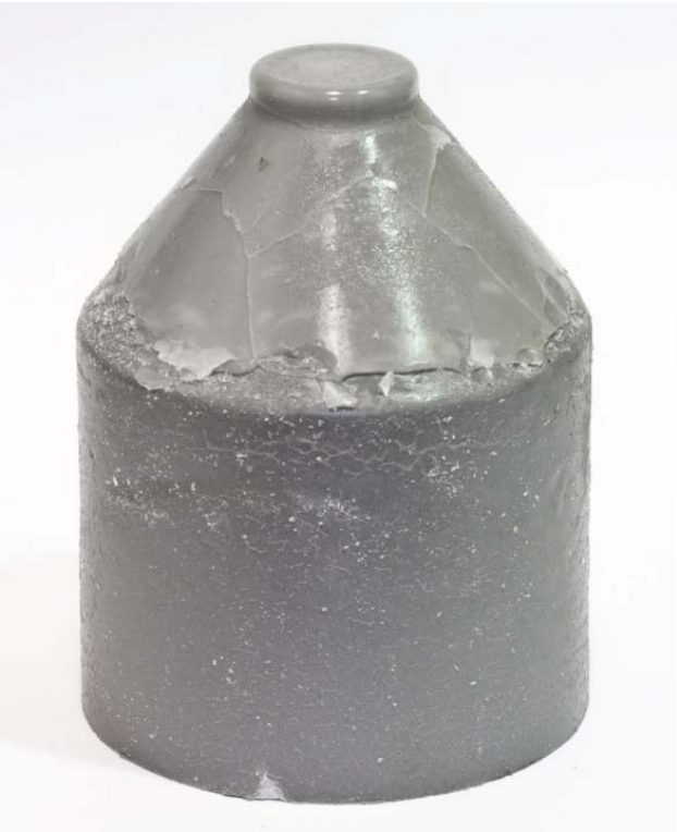
PBXN-109 Billet -Cast Configuration -Removed from case -Approx. 7 lbs N.E.W.
